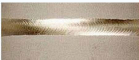
Fig 1b To ensure no discolouration occurs the oxygen content needs to be reduced to 20 ppm (0.002%).
