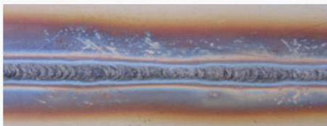
Fig 1a The result of unprotected underbead in welded austenitic stainless steel
